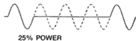
Typical Output Waveforms of Load Voltages for 3 Phase 2 LEG and 3 LEG Control
