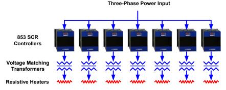
Figure 11. Typical Transformer Coupled Heating Application
